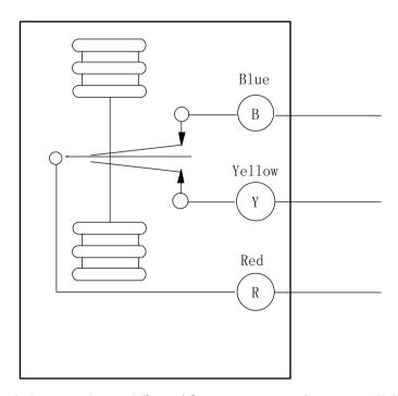
On Decrease in Pressure Differential, floating contact arm makes common RED (R) to Blue (B) Terminal On Increase in Pressure Differential, floating contact arm makes common RED (R) to Yellow(Y) Terminal
