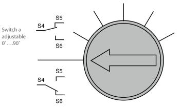
Built-in Microswitch Adjustment. Move the screw of the micro switch.
